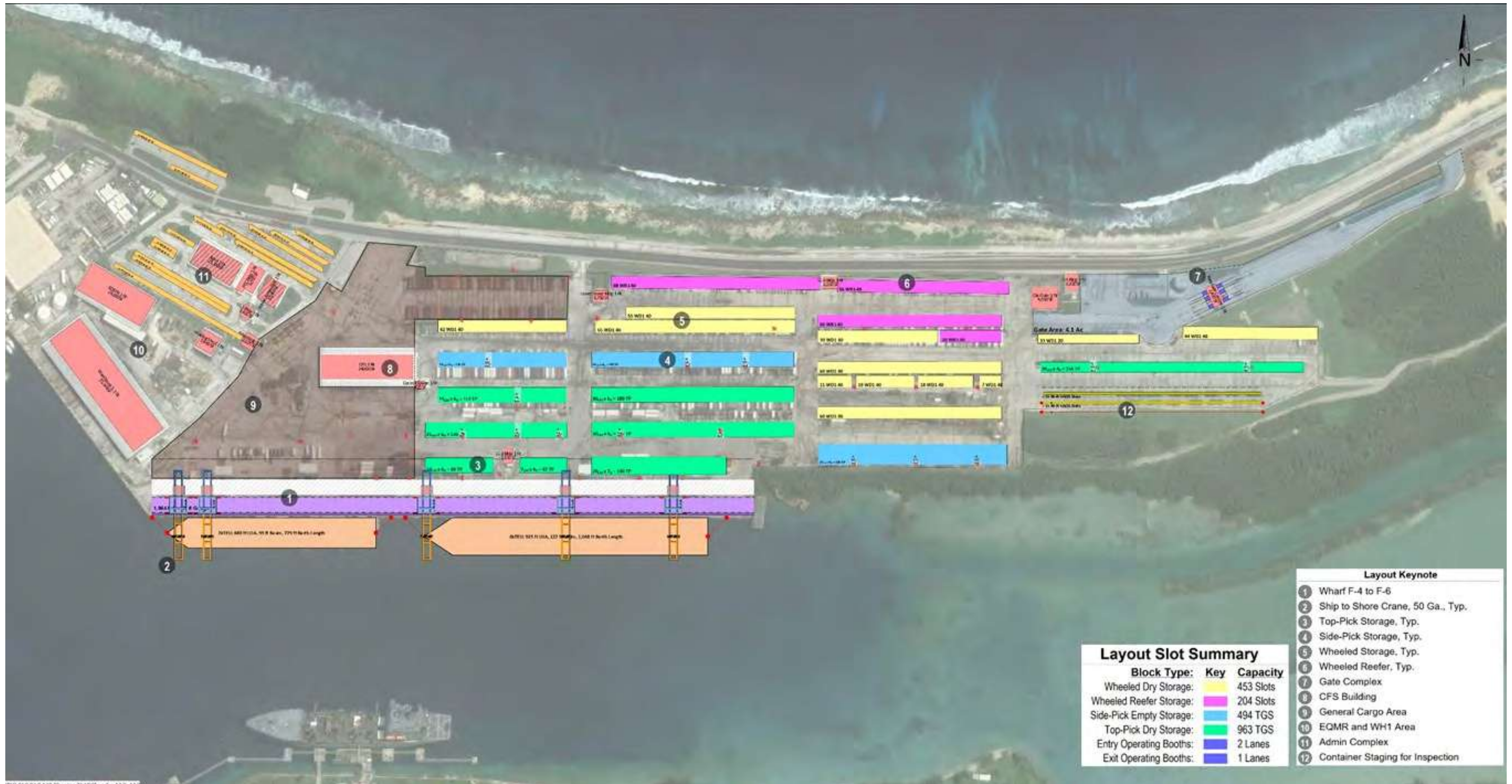
Figure 6-14: Improved Terminal Layout – Stage 2 Build-up
