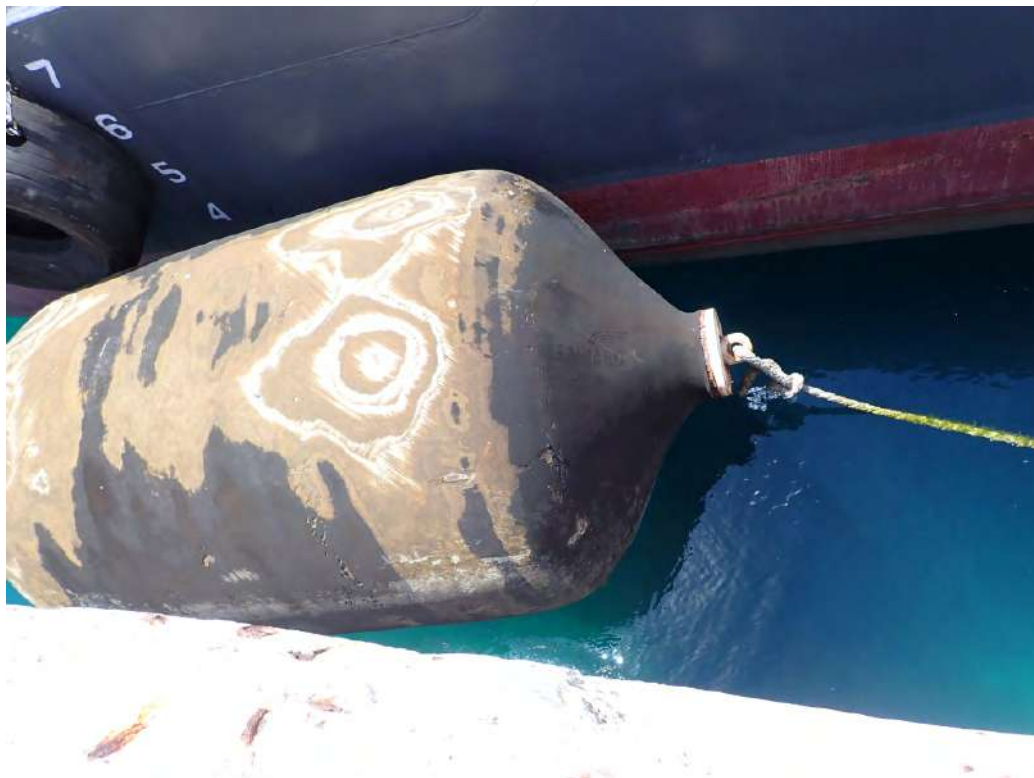
Photo 4 – Berth F2 Typical Floating Pneumatic Fender
