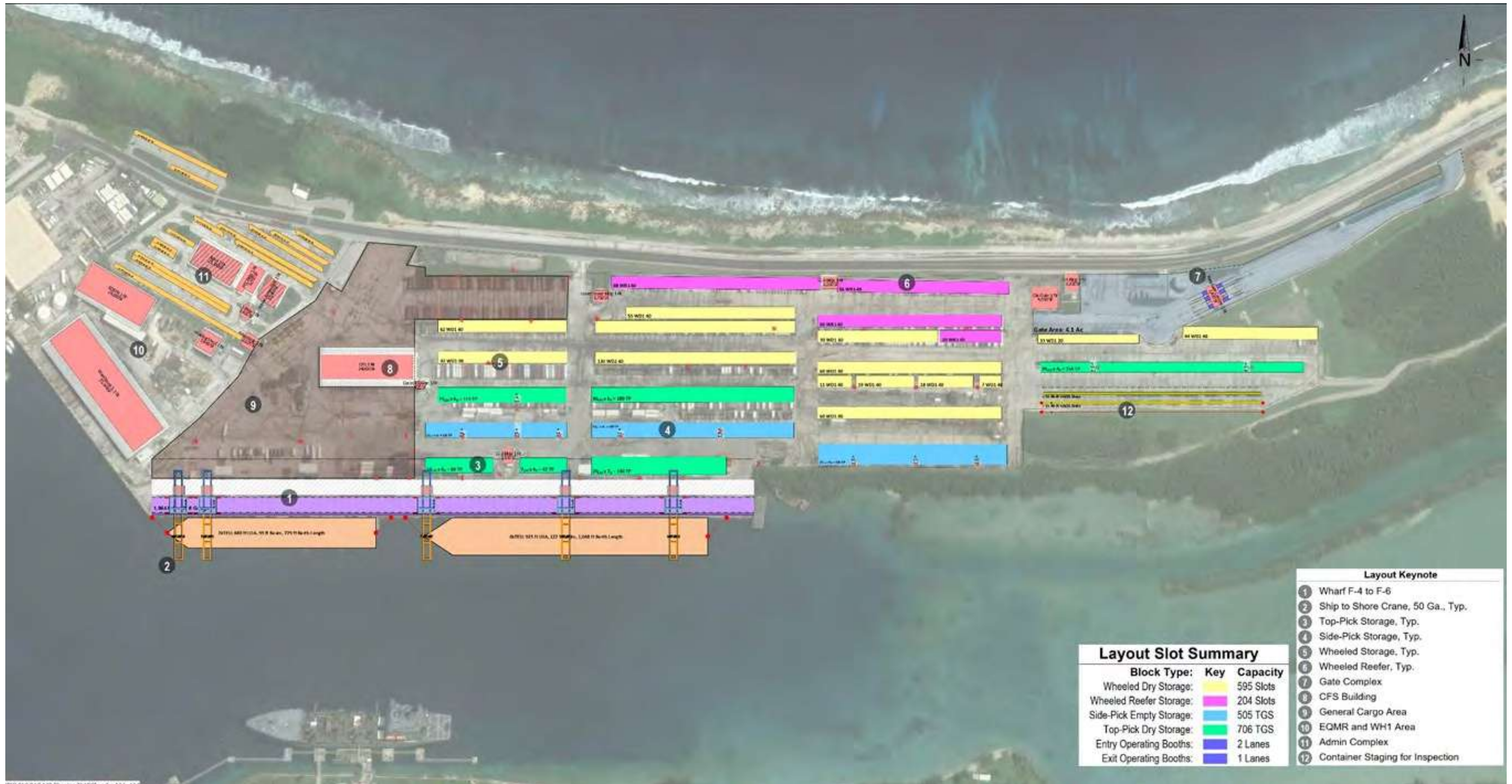
Figure 6-13: Improved Terminal Layout – Stage 1 Ramp-Up
