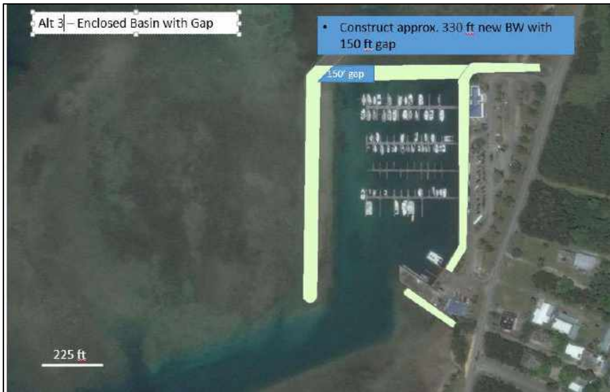
Figure 46. Agat SBH Alternative 3 – Enclosed Basin with Gap
