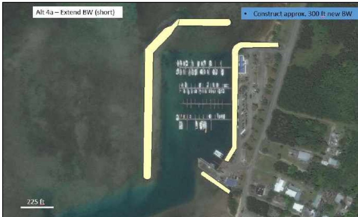
Figure 47. Agat SBH Alternative 4a – Extend Breakwater (300 ft)
