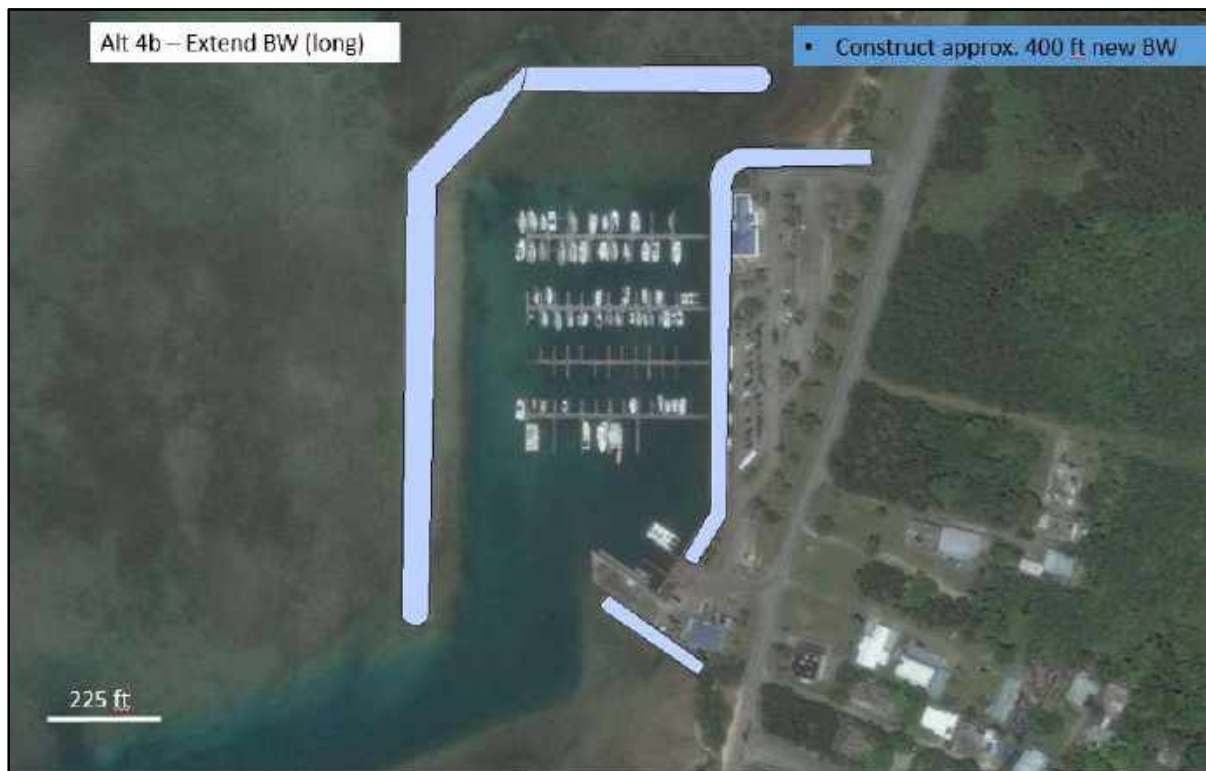
Figure 48. Agat SBH Alternative 4b – Extend Breakwater (400 ft)
