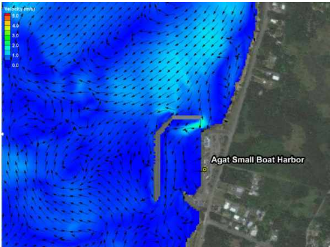
Figure 55. Alt 4a Current velocity field for annual wave condition - 7/30/09 at 12:00pm (GMT)
