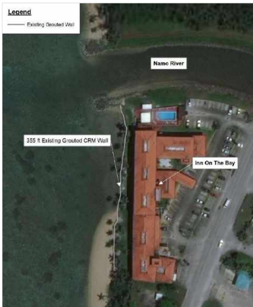
Figure 70. Location of Inn on the Bay and alignment of existing grouted CRM wall.
