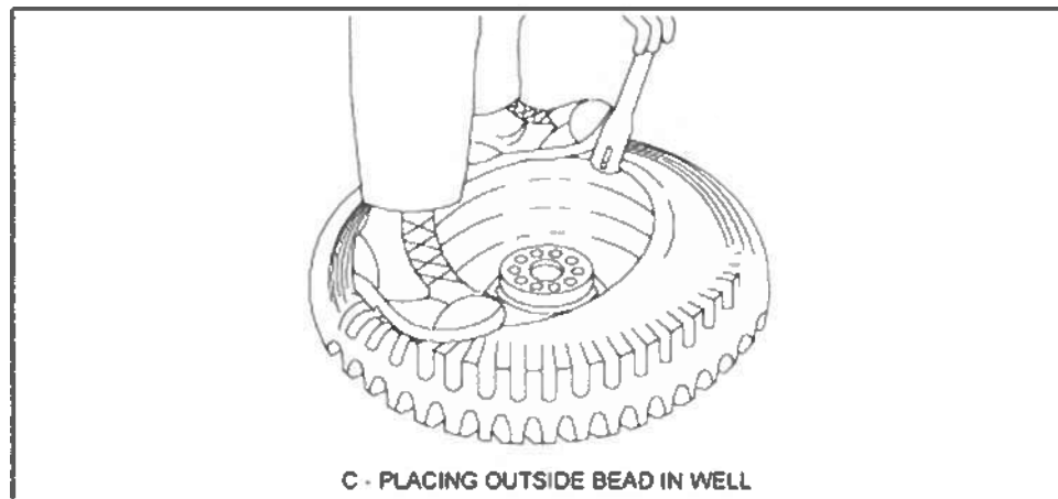
Figure 4-20. Manually Mounting Tire-Drop Center Rim
